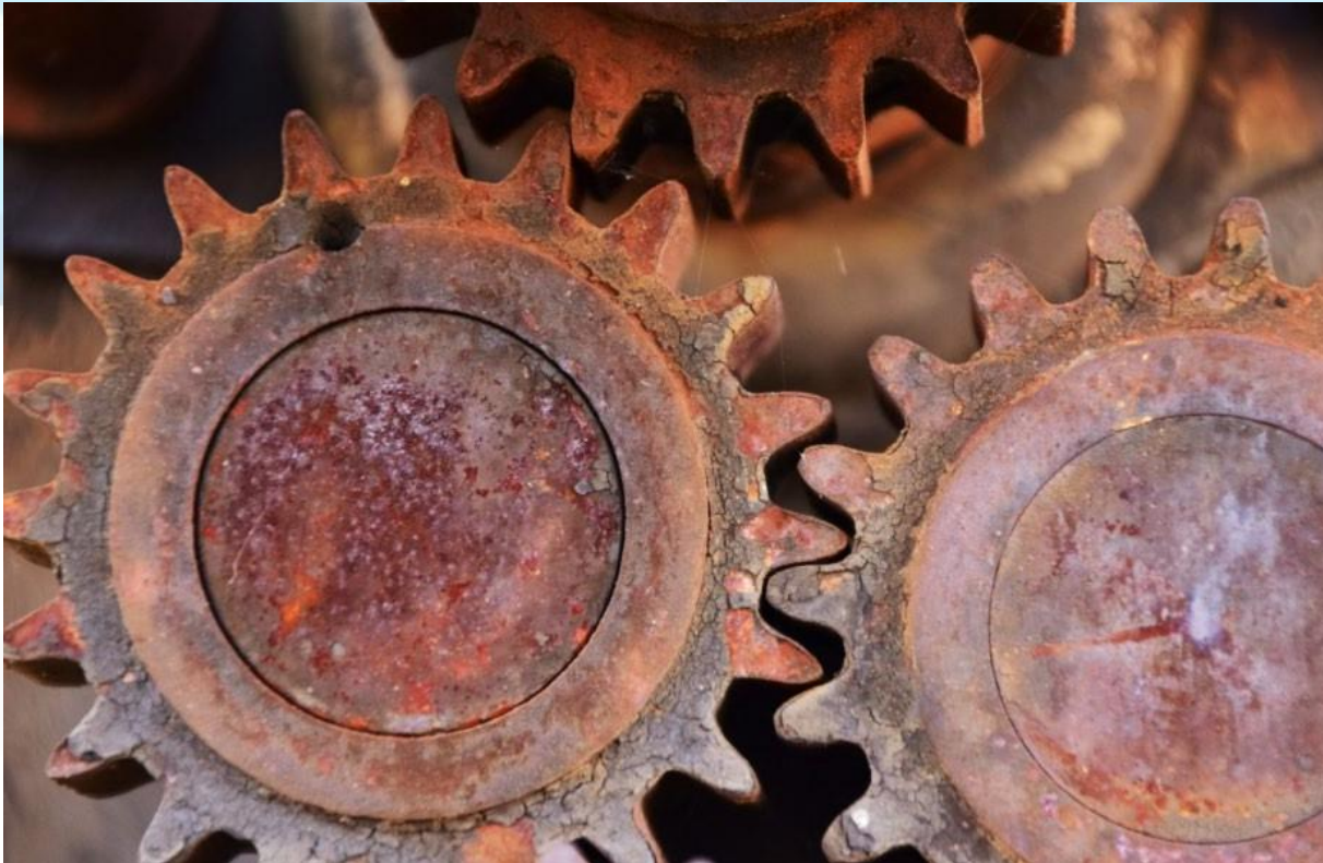
Figure 1: Gear wheels exposed to corrosion
