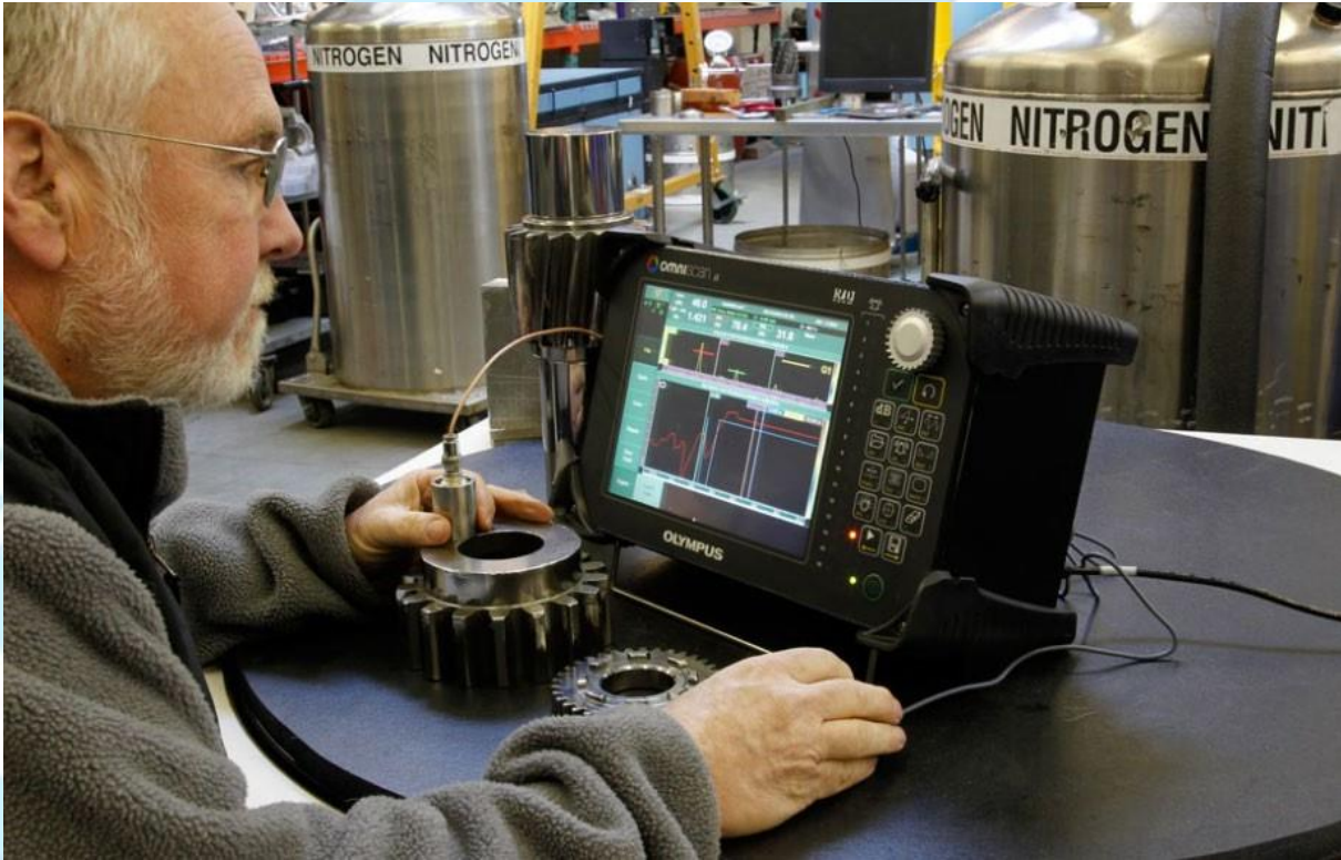
Figure 8: Application of the ultrasonic inspection method on the gear wheel
