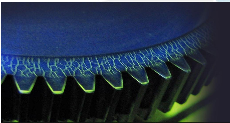
Figure 3: Application of the magnetic particle inspection method on gears
